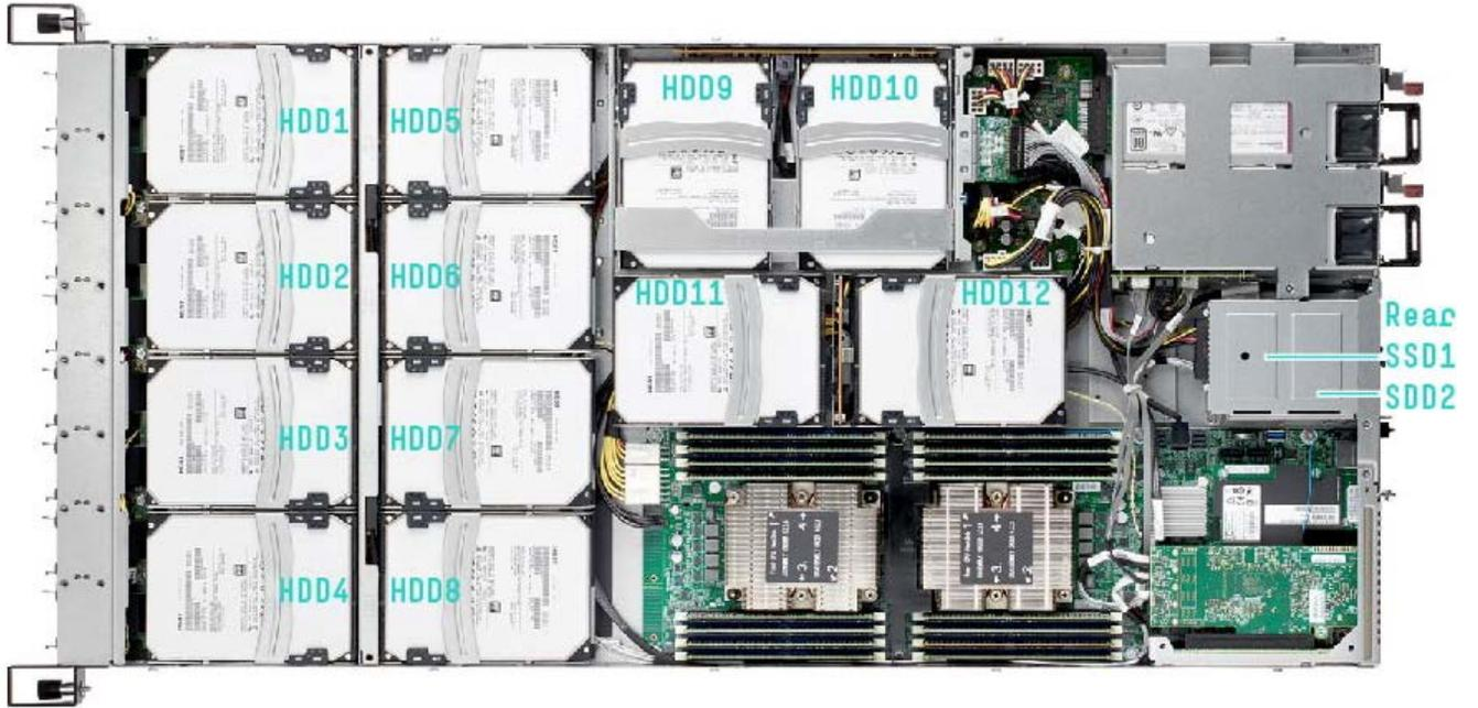
12 LFF HDDs without HDD backplane and non-HBA card
